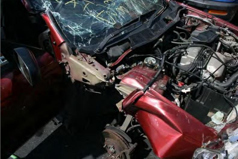
5. At the same time Horizontal relief cuts need to be made in the base of the A-post. The cuts ideally should be horizontal but only the situation will dictate where the relief cuts are made. This can be carried out earlier on before we tension a ram against the A-post
