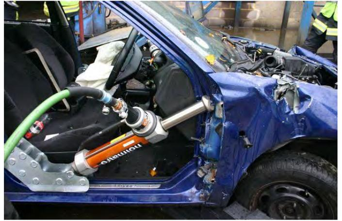
3. Once you have tension on the ram against the A-post, cut a 1-2 inch piece out of the A-post so that when we roll the dash the A-post will not catch against itself, (with skill you can angle the tool blade so that the lower post ends up on the outside of the vehicle after the cut). Or if time permits and no complications occur cut out the whole upper section of A-post completely
