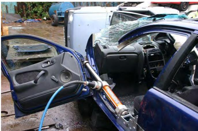
Notice how the door glass is still intact, again saving time not having to manage it, however sheeting it over would be standard procedures in case of accidental breakage.
