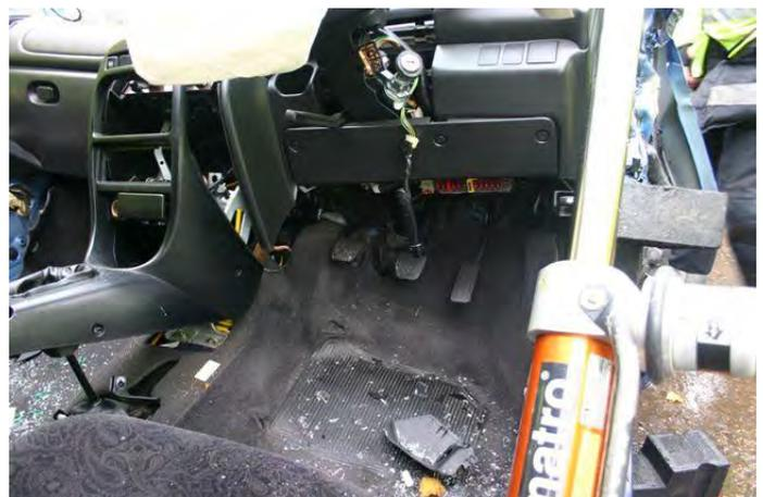
Eventually the whole engine compartment started to roll down. You can start to see the displacement of the centre console and floor plan.
