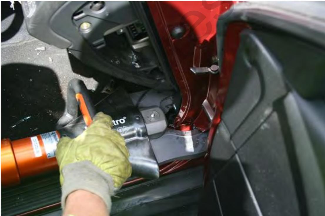
6. Once all the cuts are complete and the stabilisation has been checked, we can now think about starting to ram either against the A-post or a Door hinge, we did both on each side of the car, the side where we rammed of the door hinge, didn't effect the door glass and this stayed intact through out.
